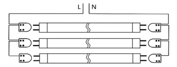
**Step 4:** Affix the field applied label to the light fixture and install the tube. The tube has double ended wiring connection.
