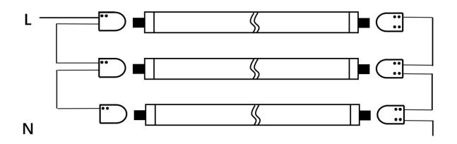
• Step 3: Affix the field applied label to the light fixture and install the tube. The tube is double ended wiring connection.
