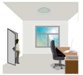
With suffcient natural light, the light does not switch on when presence is detected.
