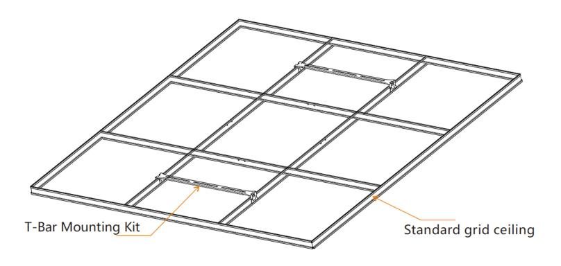
When emergency LED drivers cannot be installed on the LED lights (down lights, panels, troffers, etc.), we can install the emergency LED drivers on the T-bars which are installed on the grid ceiling.
