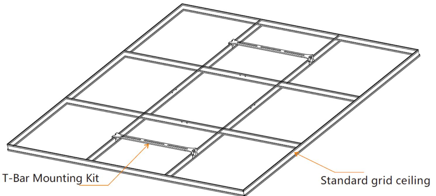
When emergency LED drivers cannot be installed on the LED lights (down lights, panels, troffers, etc.), we can install the emergency LED drivers on the T-bars which are installed on the grid ceiling.
