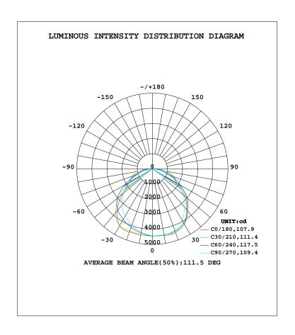
C Range: 0 - 360DEG C Interval: 15.0DEG Test Speed: HIGH Temperature: 0.0DEG Operators:Zhuwz  $\begin{array}{lll} \gamma & \text{Range:} & 0 & \text{-} & 180\text{DEG} \\ \gamma & \text{Interval:} & 0.5\text{DEG} \end{array}$
