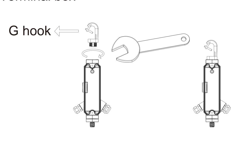
2:Fix the junction box on the lamp with a wrench
