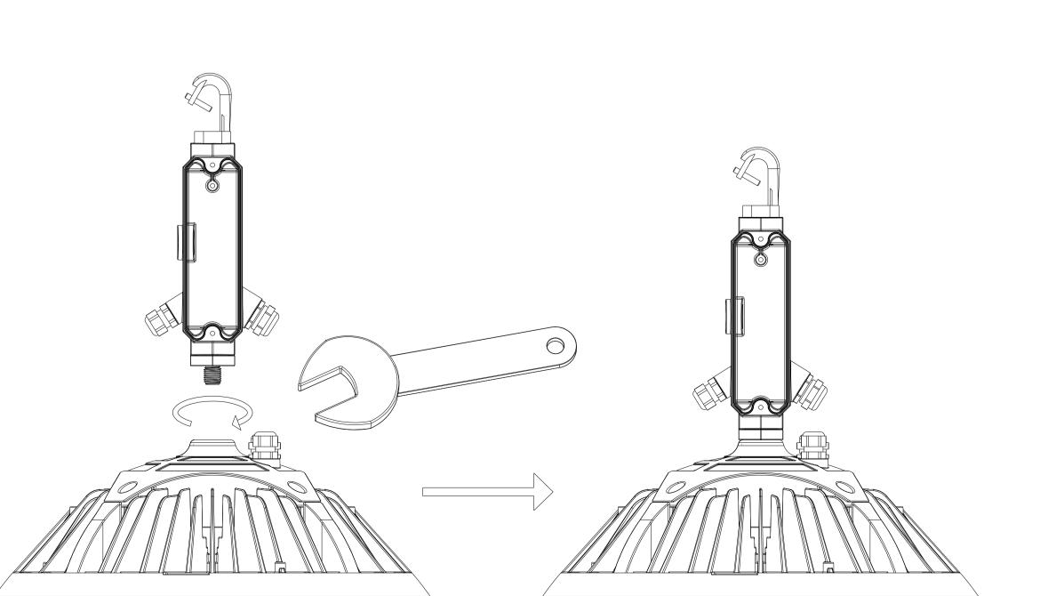
3:First, install the emergency power supply and g-hook on the hook respectively. After safety wiring, fix the upper cover of the junction box with tools
