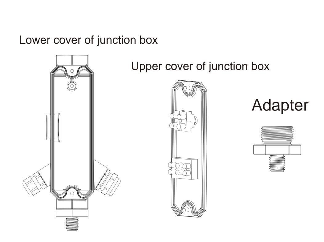
1:Use a wrench to fix the lower cover of the adapter box on the 3 / 4 American threaded pipe
