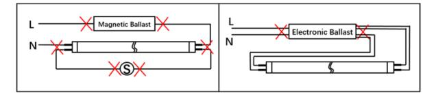
• Step 3: Install the LED tube and make the electrical connection.
