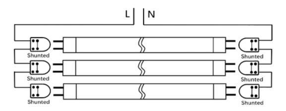
• Step 4: Affix the field applied label to the light fixture and install the tube. The tube has single end wiring connection. There are descriptions of connections for the source of electrical supply to the lamp pins. Please make sure no wiring connection on the other end.
