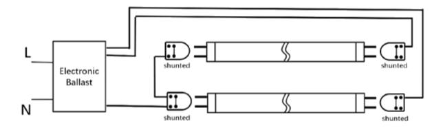
**Type B (ballast by-pass) (double end):** To replace the traditional fluorescent tube, please reconnect the electric circuit. Please check the connection instruction image as follows:
