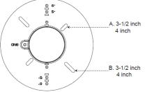
3-1/2 inch & 4 inch for Junction box5 inch & 6 inch for Recessed housing
