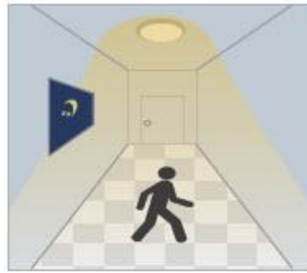
With insufficient daylight, when motion detected, light ON.
