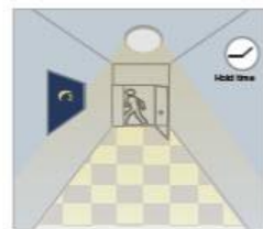
After last detection, the light will be dimmed down to the stand-by dimming level (10%, 20%,30% or 50%) after holdtime.
