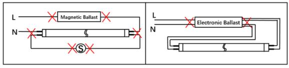
• Step 3: Install the LED tube and make the electrical connection.
