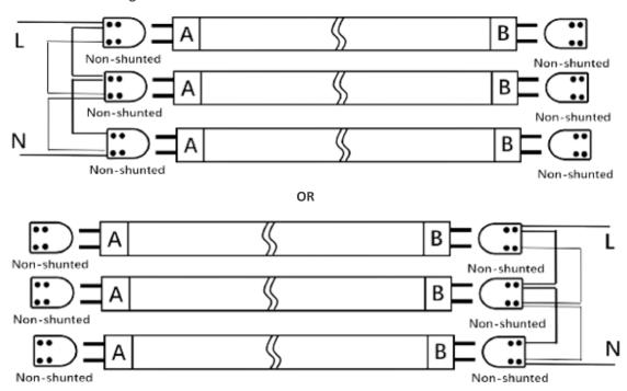
• Step 4: Affix the field applied label to the light fixture and install the tube. The tube has single end wiring connection. There are descriptions of connections for the source of electrical supply to the lamp pins. Please make sure no wiring connection on the other end.
