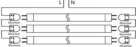
Step 4: Affix the field applied label to the light fixture and install the tube. The tube has double ended wiring connection.
