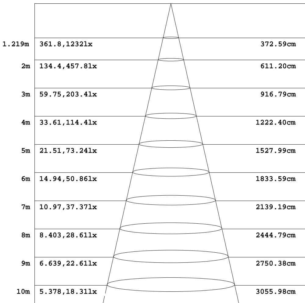
Height      Eavg ,Emax      Angle:113.59deg      Diameter
